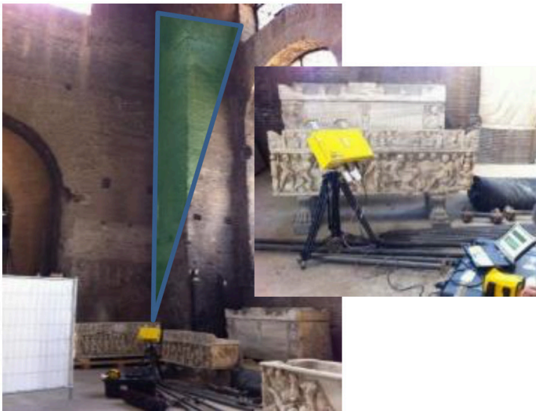
Figure 16. Radar interferometry measurements, the south pillar of Hall I.
