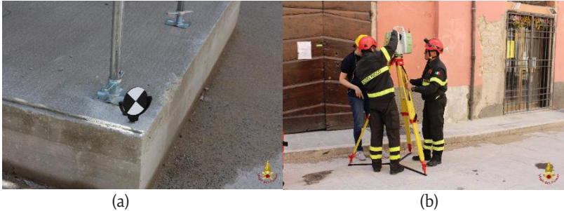
Figure 31. Example of checkerboard targets (a) in a Laser scanning session in Norcia (Italy) undertaken by the Italian Fire Fighters (b) after a strong earthquake.
